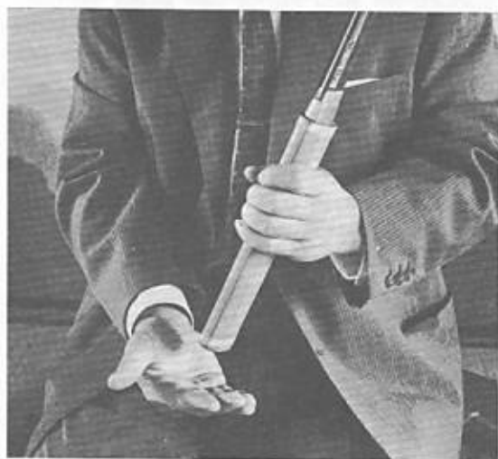
(8) Fixing a tang in the hilt after oiling
